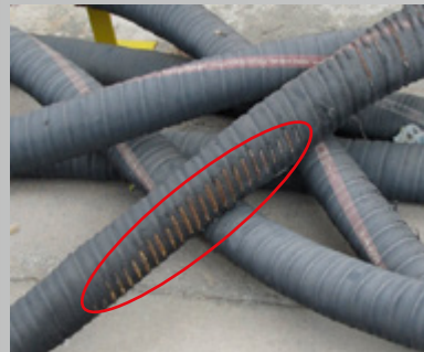
Exposed wire seen on chemical hose due to severe abrasion or chemical exposure.
