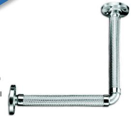
Uncontrolled movements are best addressed with a construction that can fully accommodate multiple movements. A dogleg hose is really two complete assemblies that are joined by an elbow, which combines their flexibility and allows the assembly to go a combination of up, down, and side-to-side. To reduce the number of leak points and increase the overall flexible length of the hose, Hose Master employs expertly trained welders to make these hoses a fully-welded assembly.
