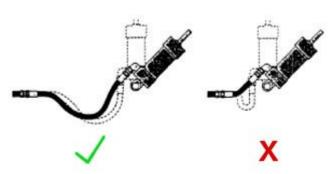
**5.23.2 – Hose and Machine Tolerances –** Design hose to allow for changes in length due to machine motion and tolerances.
