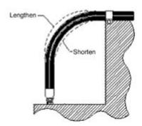
**5.24 – Hose Movement and Bending –** Hose allows relative motion between system components. Analyze this motion when designing hose systems.
