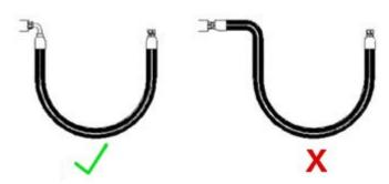
5.23 - Lengths - Unnecessarily long hose can increase pressure drop and affect system performance. When pressurized, hose that is too short may pull loose from its fittings, or stress the fitting connections, causing premature metallic or seal failures.
