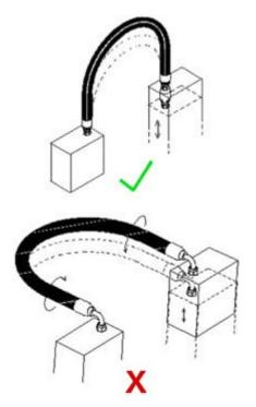
**5.24.2** – **Prevent Hose Bending in More Than One Plane** – if the hose follows a compound bend, couple it into separate segments that flex only in one place.
