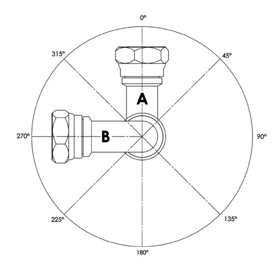
Orientation is determined by the number of degrees measured in a clockwise direction between the farthest fitting and the nearest fitting.
